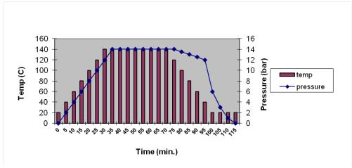
Above is an example of a typical autoclave pressure/temperature/time cycle. Actual pressures and temperatures can vary to some degree, but the shape of the curve will be similar in close to 100% of the cases.
