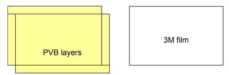
Steps 2 & 3: Align interlayer films onto glass (PVB/3M film/PVB). Align second piece of glass
